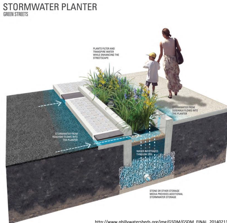
Figure 2. Example schematic of green street stormwater capture (from Philadelphia Green Street Design Manual)
